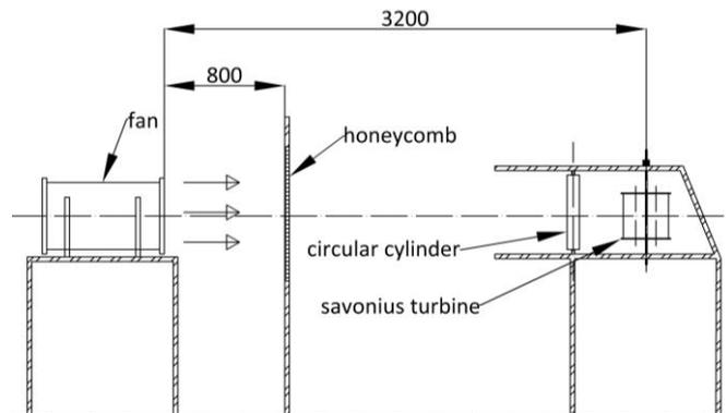
**Fig. 2.** Arrangement diagram of the experiment
