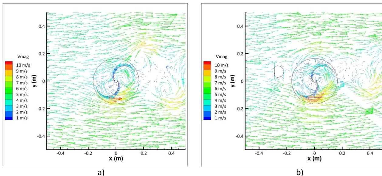
**Fig. 8.** Velocity vector of fluid around the turbine  $\theta = 30^\circ$ ,  $\lambda = 0.6$  at Reynolds number = 95,000; (a) without passive control cylinder (b) with passive control cylinder.
