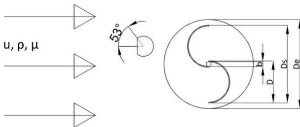
**Fig. 1.** Schematic diagram of the Savonius turbine and the passive control cylinder
