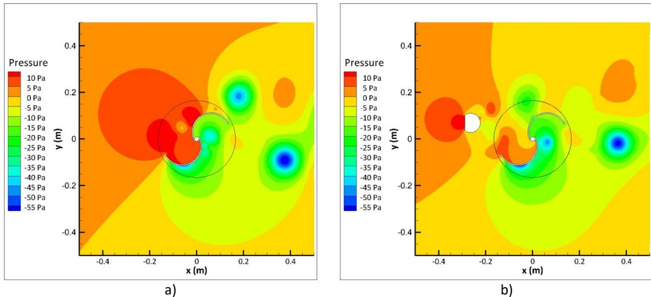
**Fig. 7.** Pressure contour of fluid around the turbine  $\theta = 30^\circ$ ,  $\lambda = 0.6$  at Reynolds number = 95,000; (a) without passive control cylinder (b) with passive control cylinder.
