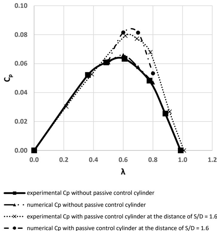
**Fig. 5.** Comparison of  $C_p$  between turbine with and without passive control cylinder
