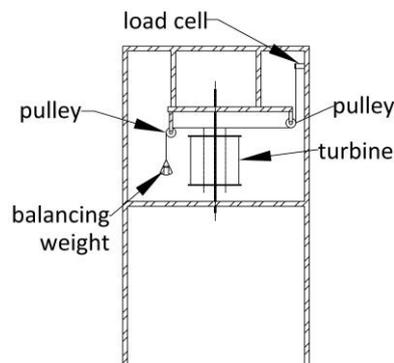
**Fig. 3.** Rope brake dynamometer system
