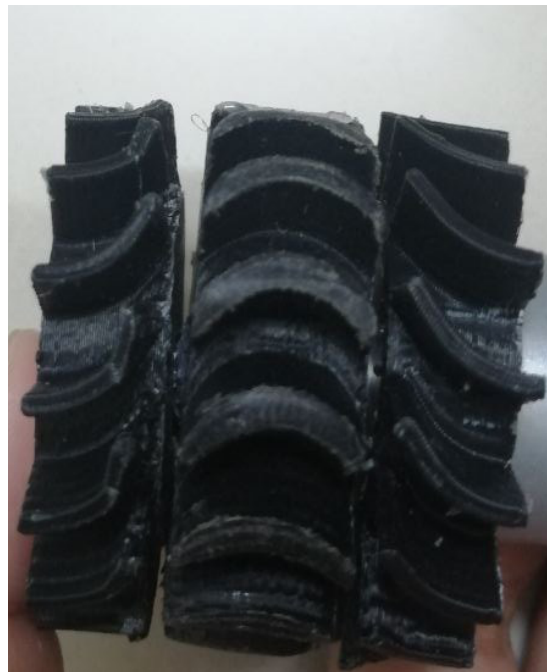
Fig. 2. The assembled 3D printed stator on the left (upstream), the rotor in the middle and the stator on the right (downstream)
