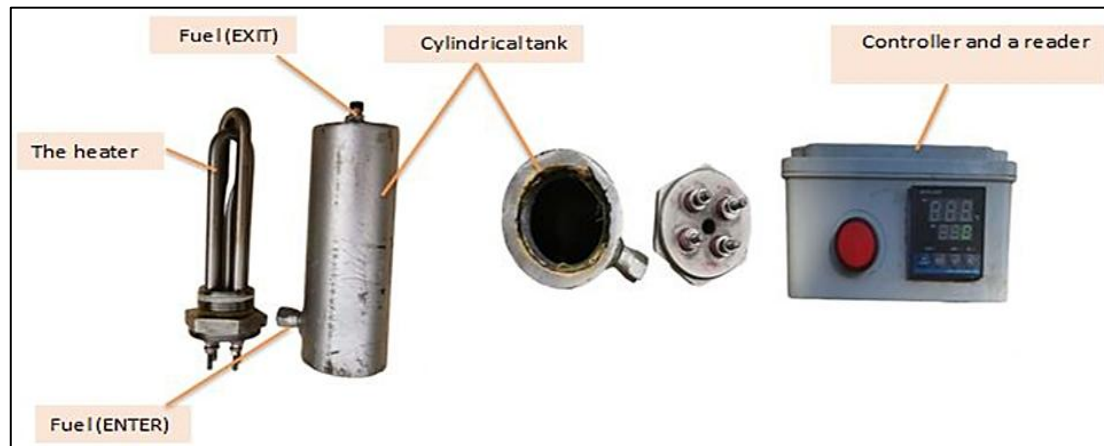
Fig. 3. Fuel heater system
