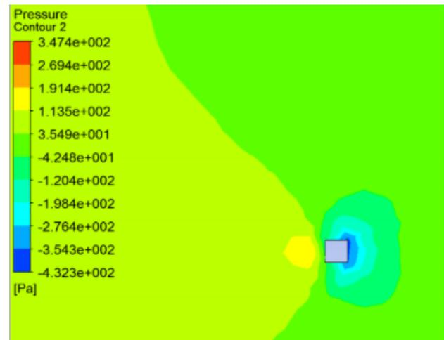
(b) Pressure Values at Fluid Velocity 30 m/s
