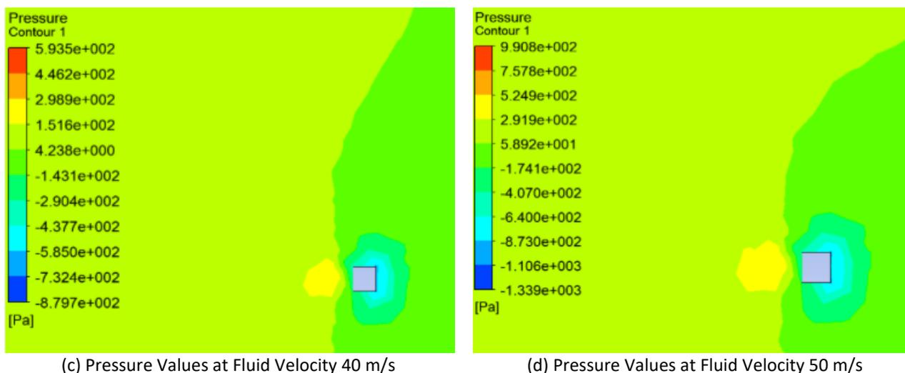
**Fig. 6.** Pressure contours of fluid striking rooftop at 60°
