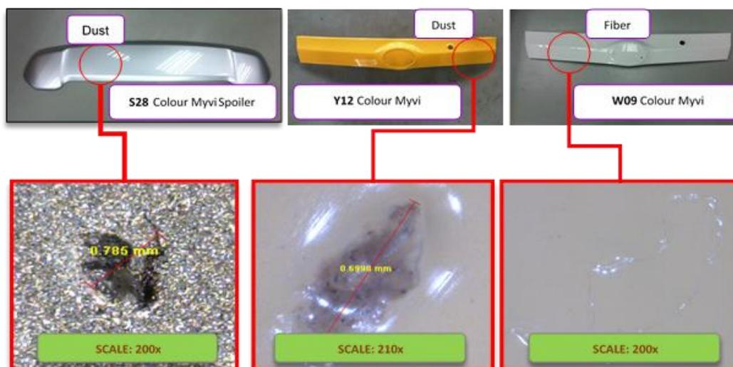
Fig. 2. Source of contamination of dust and in painting line [1]
