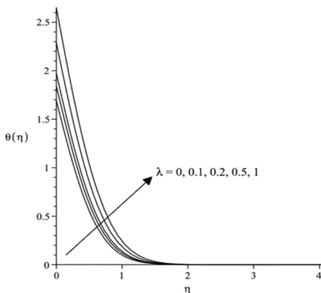
**Fig. 4.** Effect  $\lambda$  on  $\theta(\eta)$  when  $Pr=6.2$ ,  $\varepsilon=0.5$ ,  $\gamma=M=1$  and  $\varphi=0.1$ .
