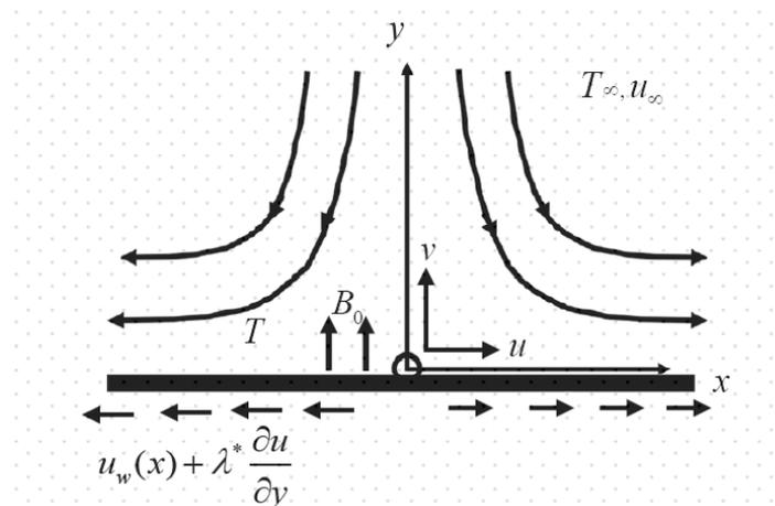
Fig. 1. Physical model and the coordinate system
