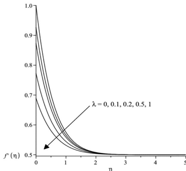
**Fig. 7.** Effect  $\lambda$  on  $f'(\eta)$  when  $Pr=6.2$ ,  $\varepsilon=0.5$ ,  $\gamma=M=1$  and  $\varphi=0.1$ .
