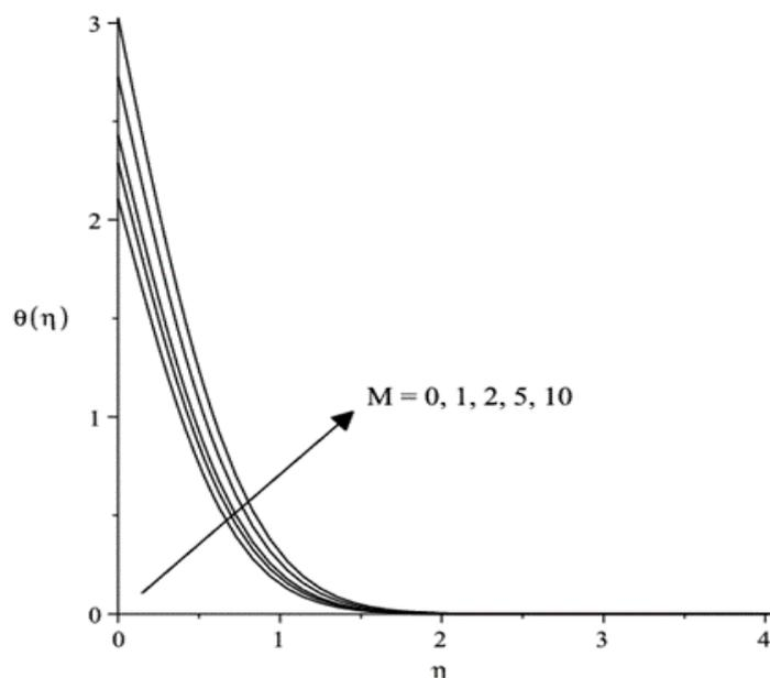
**Fig. 3.** Effect  $M$  on  $\theta(\eta)$  when  $Pr=6.2$ ,  $\varepsilon=\lambda=0.5$ ,  $\gamma=1$  and  $\varphi=0.1$ .
