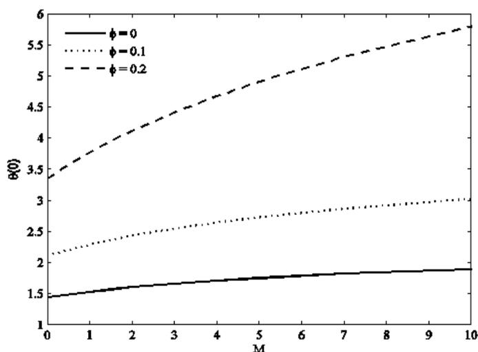
**Fig. 8.** Effect  $M$  and  $\varphi$  on variation of  $\theta(0)$  when  $Pr=6.2$ ,  $\varepsilon=\lambda=0.5$  and  $\gamma=1$ .
