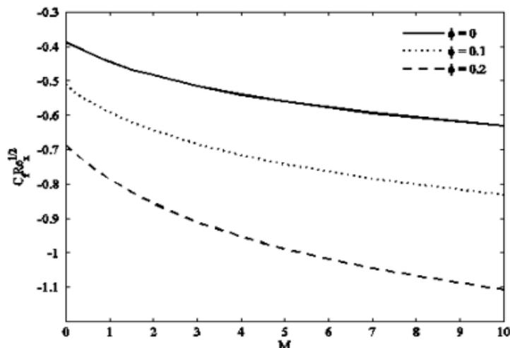
Fig. 9. Effect  $M$  and  $\phi$  on variation of  $C_f Re_x^{1/2}$  when  $Pr = 6.2$ ,  $\varepsilon = \lambda = 0.5$  and  $\gamma = 1$ .
