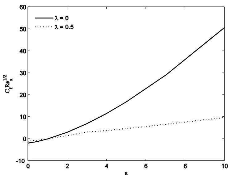
Fig. 10. Effect  $\varepsilon$  and  $\lambda$  on variation of  $C_f Re_x^{1/2}$  when  $Pr = 6.2$ ,  $M = 1$ ,  $\phi = 0.1$  and  $\gamma = 1$ .
