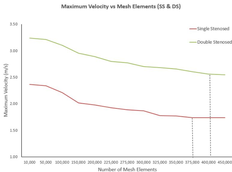
**Fig. 1.** Mesh Dependency for SS and DS
