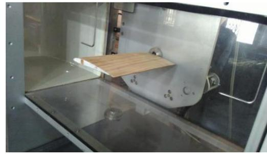
(b) NACA 7037 Airfoil made of Kale wood
