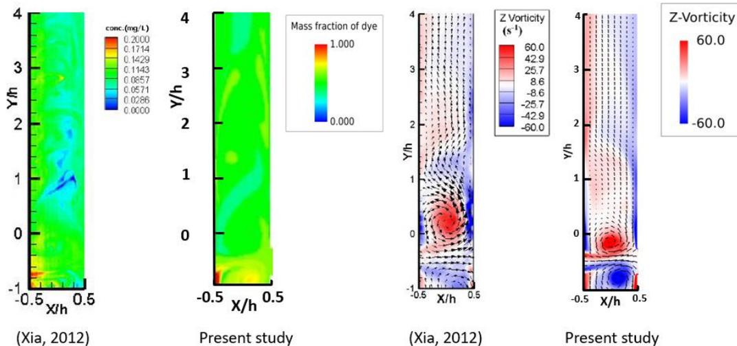
**Fig. 13.** Comparison between instantaneous concentration contours (left), and phase-averaged velocity vector and vorticity contours (right) obtained from experiment and present study. All the visualization results are captured near the orifice exit region at the end of ejection cycle of left SJA under stroke ratio,  $L = 8$  and velocity ratio,  $R_v = 3.2$
