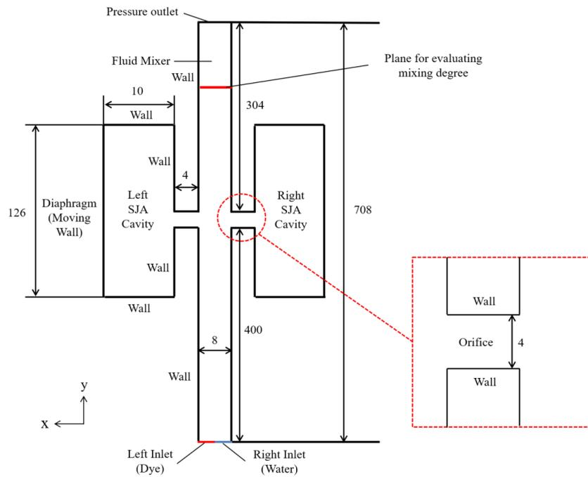
**Fig. 1.** 2D Schematic diagram of the geometric model
