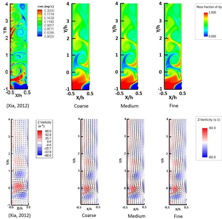
**Fig. 5.** Comparison of instantaneous concentration contours (upper), and phase-averaged velocity fields and vorticity contours (bottom) among experiment and three difference meshes. All the visualization results are captured around the orifice exit region at the end of ejection cycle of left SJA under stroke ratio,  $L = 4$  and velocity ratio,  $R_v = 1.6$
