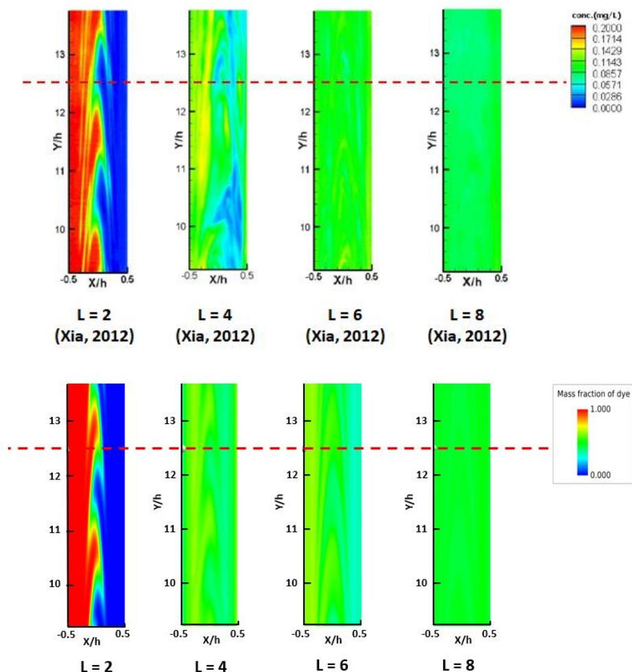
**Fig. 14.** Instantaneous concentration contours around the evaluation plane region (indicated by red dot line) shown by experiment [16] (upper), and present study (bottom) at different stroke ratios,  $L = 2, 4, 6$  and  $8$ , which corresponded to  $R_v = 0.8, 1.6, 2.4$  and  $3.2$
