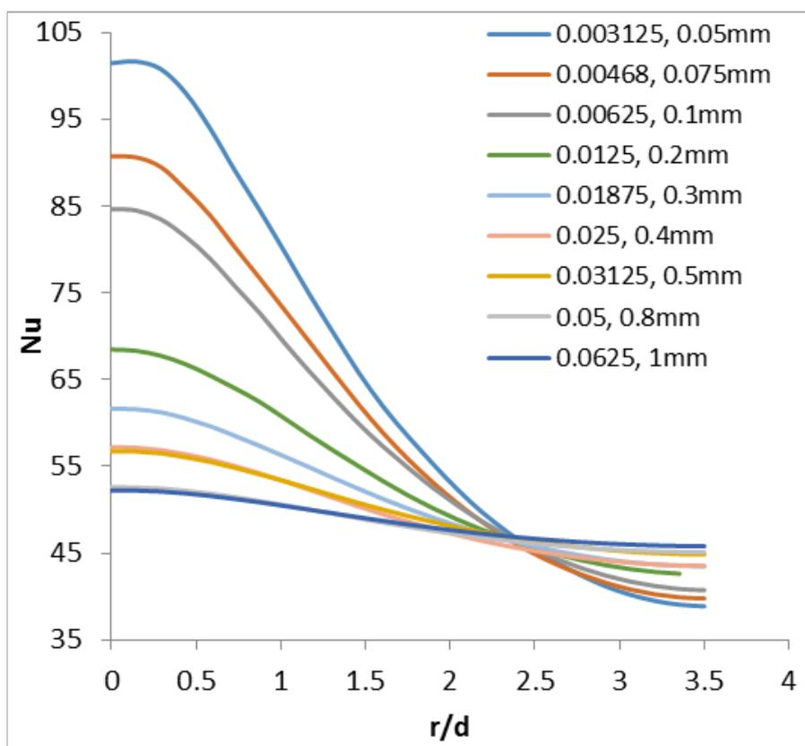
**Fig. 5.** Justifies the dependency of local Nusselt profile for different thickness of flat surface on Nozzle-target spacing  $Z/d = 6$ ,  $Re = 5000$ .
