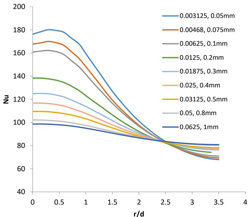
**Fig. 4.** Justifies the dependency of local Nusselt profile for different thickness of flat surface on Reynolds number  $Z/d = 4$ ,  $Re = 15000$
