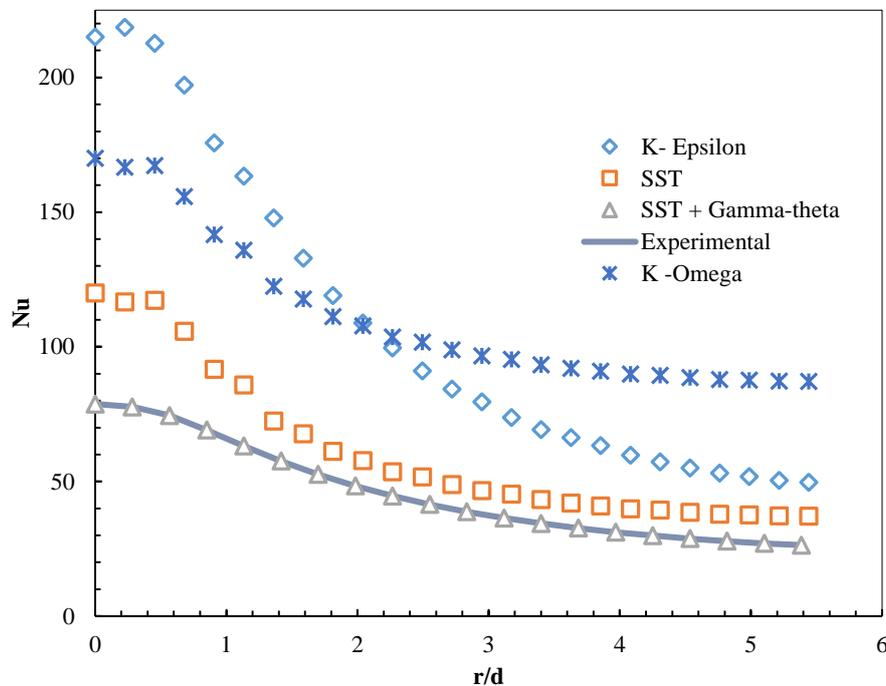
Fig. 3. Nusselt profile for different turbulence model at  $Z/d=4$ ,  $Re=6000$
