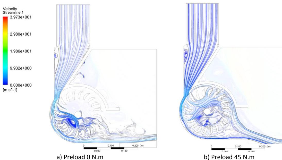
**Fig. 5.** Streamline on different preload acting on its blade
