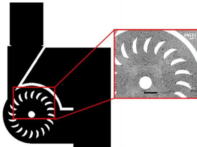
Fig. 2. 2D Domain mesh visualization – 122408 elements
