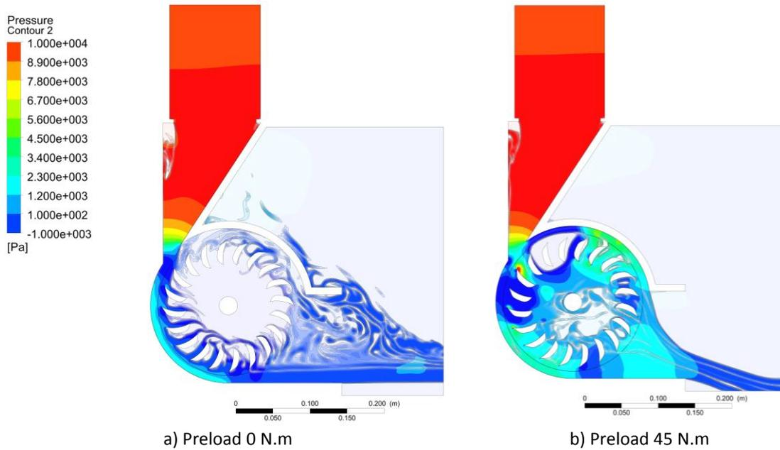
**Fig. 4.** Pressure contour on different preload acting on its blade
