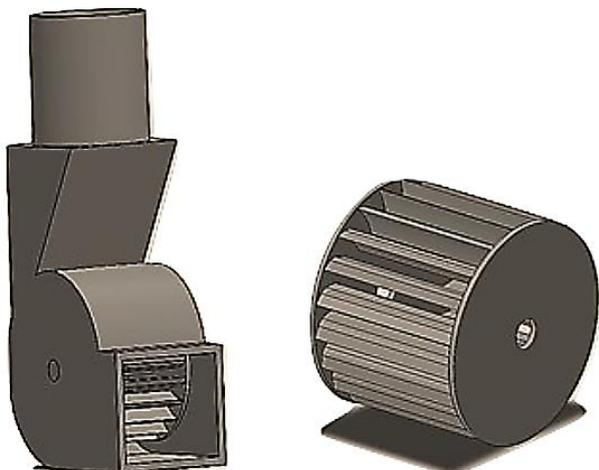
Fig. 1. 3D model of the cross-flow turbine
