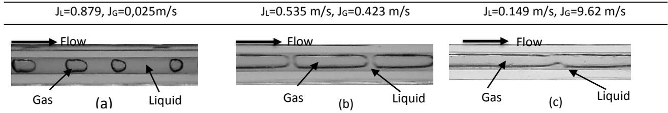
**Fig. 2.** A typical two-phase flow pattern based on  $J_L$  and  $J_G$  variations, (a) Bubble, (b). Plug, (c). Slug annular/Annular
