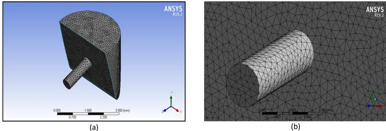
**Fig. 3.** Meshing process for internal parts in the actuator nozzle (a) Meshed model of the nozzle (b) Details view for the orifice diameter in the actuator nozzle
