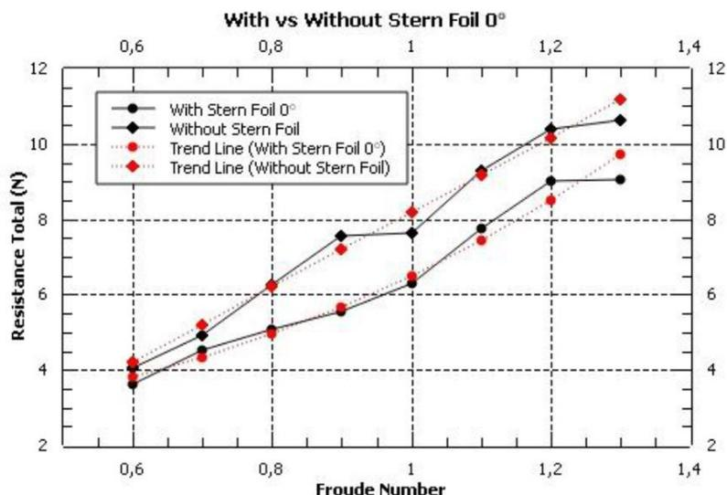
Fig. 9. Comparison application of stern foil using 0 ° angle
