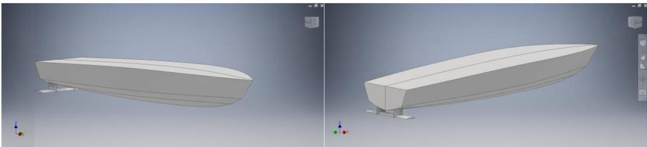
**Fig. 3.** Configuration of stern foil on the transom of Patrol hull
