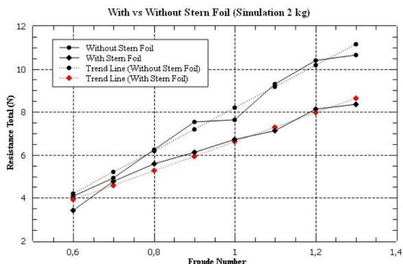
Fig. 10. Comparison application of stern foil using 3 ° angles
