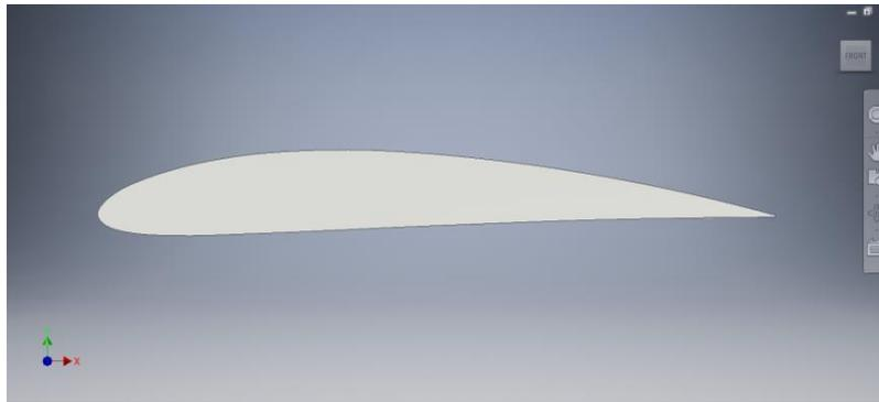
**Fig. 2.** Side view hydrofoil NACA 4412
