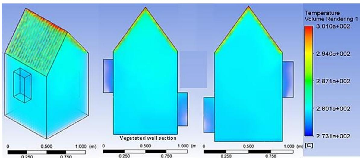
Fig. 5. Simulation result of vegetated wall model
