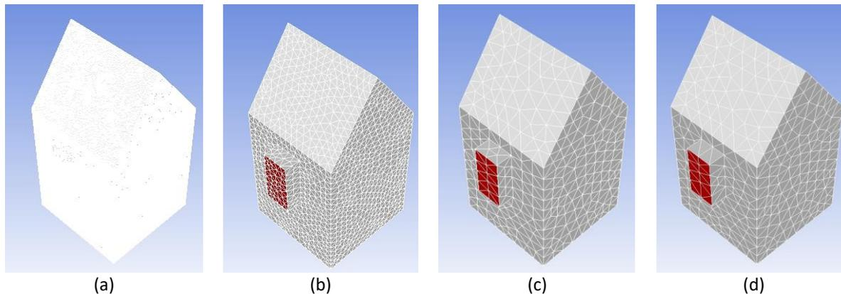
**Fig. 3.** Grid independence test of CFD simulation: (a). Meshing with grid size at 0.01 m; (b). Meshing with grid size at 0.05 m; (c). Meshing with grid size at 0.1 m; (d). Meshing with grid size at 0.5 m
