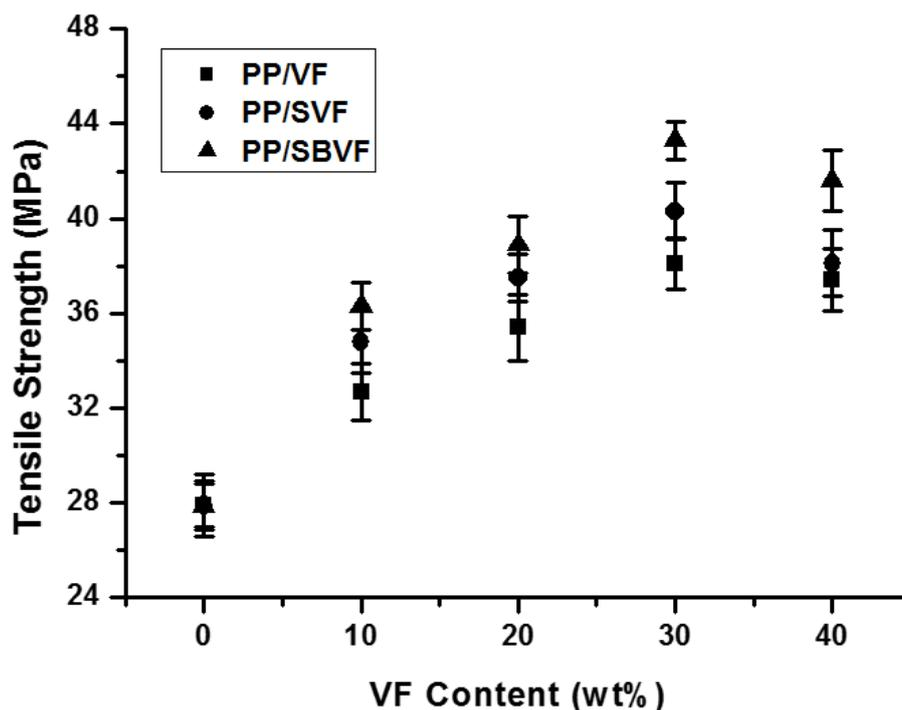
Fig. 1. Tensile strength of varied fiber loadings in PP/VF, PP/SVF, and PP/SBVF composites
