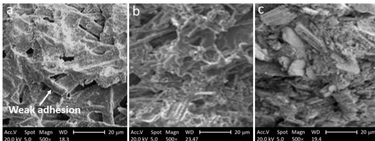
**Fig. 6.** SEM micrographs of the fracture surfaces of (a) untreated (PP/VF), (b) treated-PP/SVF, and (c) PP/SBVF composite at 30 wt% fiber content
