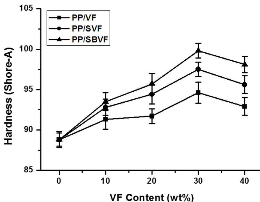
Fig. 5. Hardness of composites made of PP/VF, PP/SVF, and PP/SBVF at various fiber contents
