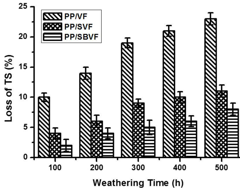
Fig. 8. Loss of tensile strength of the treated and untreated composites as a result of the weather simulation
