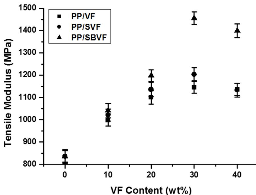
Fig. 2. Tensile modulus of composites made of PP/VF, PP/SVF, and PP/SBVF at various fiber loading
