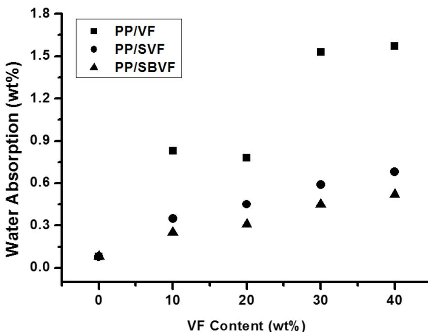
**Fig. 7.** WA values of PP/VF, PP/SVF, and PP/SBVF composites against various fiber loading as a function of water soaking period (24 h)
