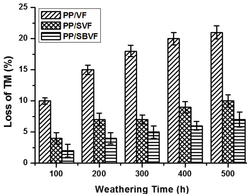
Fig. 9. Loss of tensile modulus of the treated and untreated composites as a result of the weather simulation
