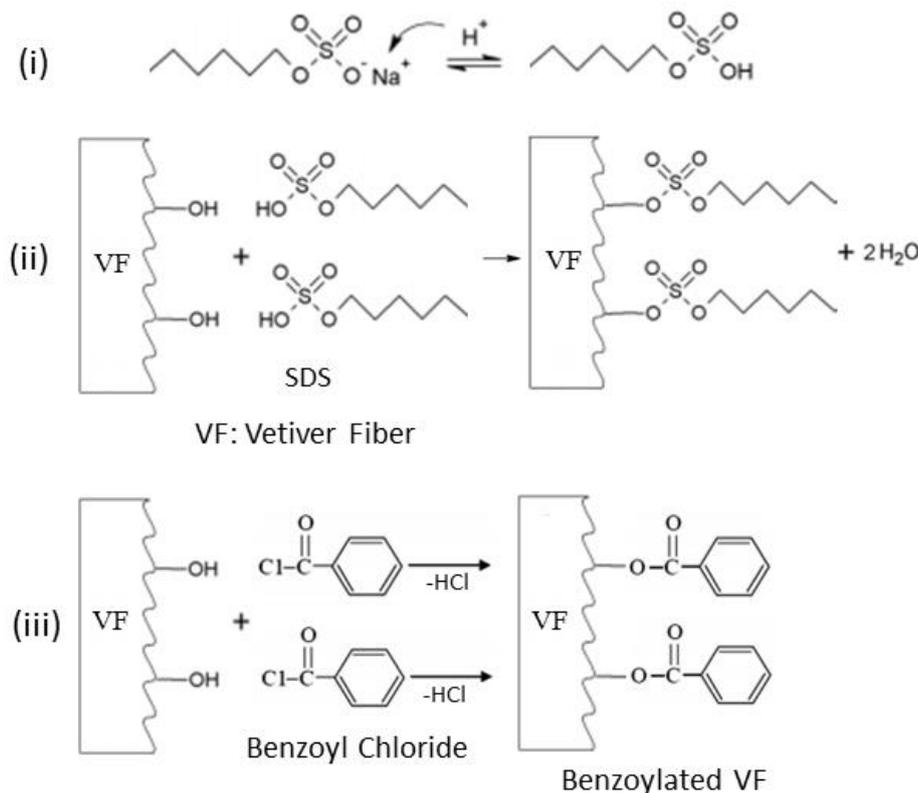
**Fig. 3.** Suggested mechanisms for the reactions of VF with sodium dodecyl sulfate (i & ii) and VF with benzoyl chloride are presented (iii)
