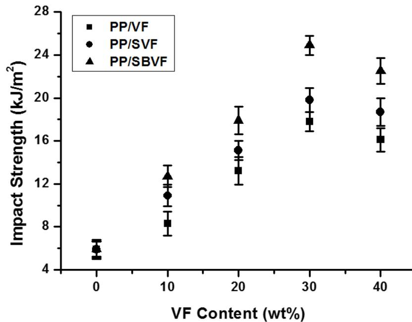
Fig. 4. Impact strength of composites made of PP/VF, PP/SVF, and PP/SBVF at various fiber contents
