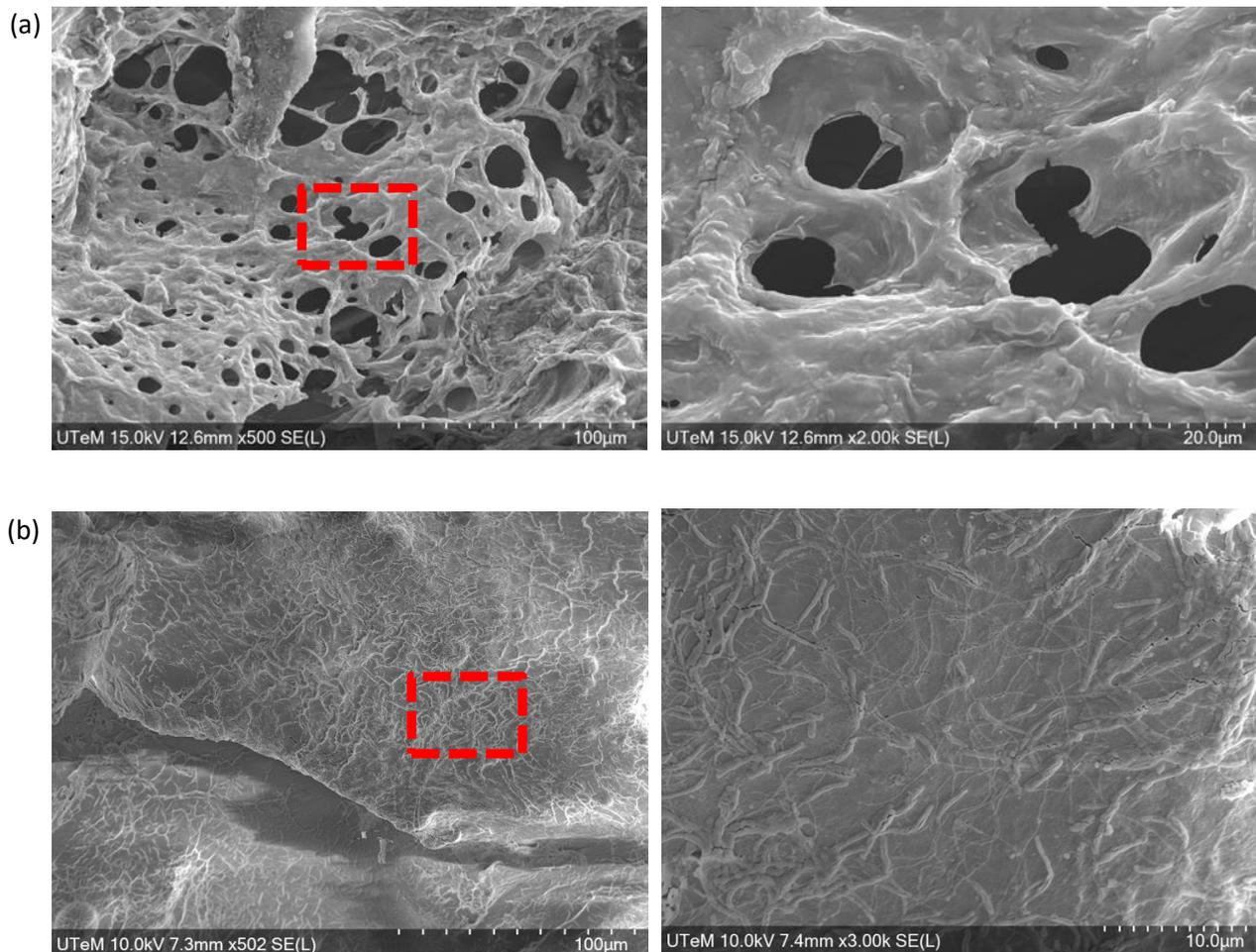
**Fig. 6.** (a) SEM imaging with magnifications of 500x (left) and 2000x (right) on the cross-section of grid square scaffold with highly porous structure, (b) SEM imaging with magnifications of 500x (left) and 3000x (right) on cross-section with shrinkage structure
