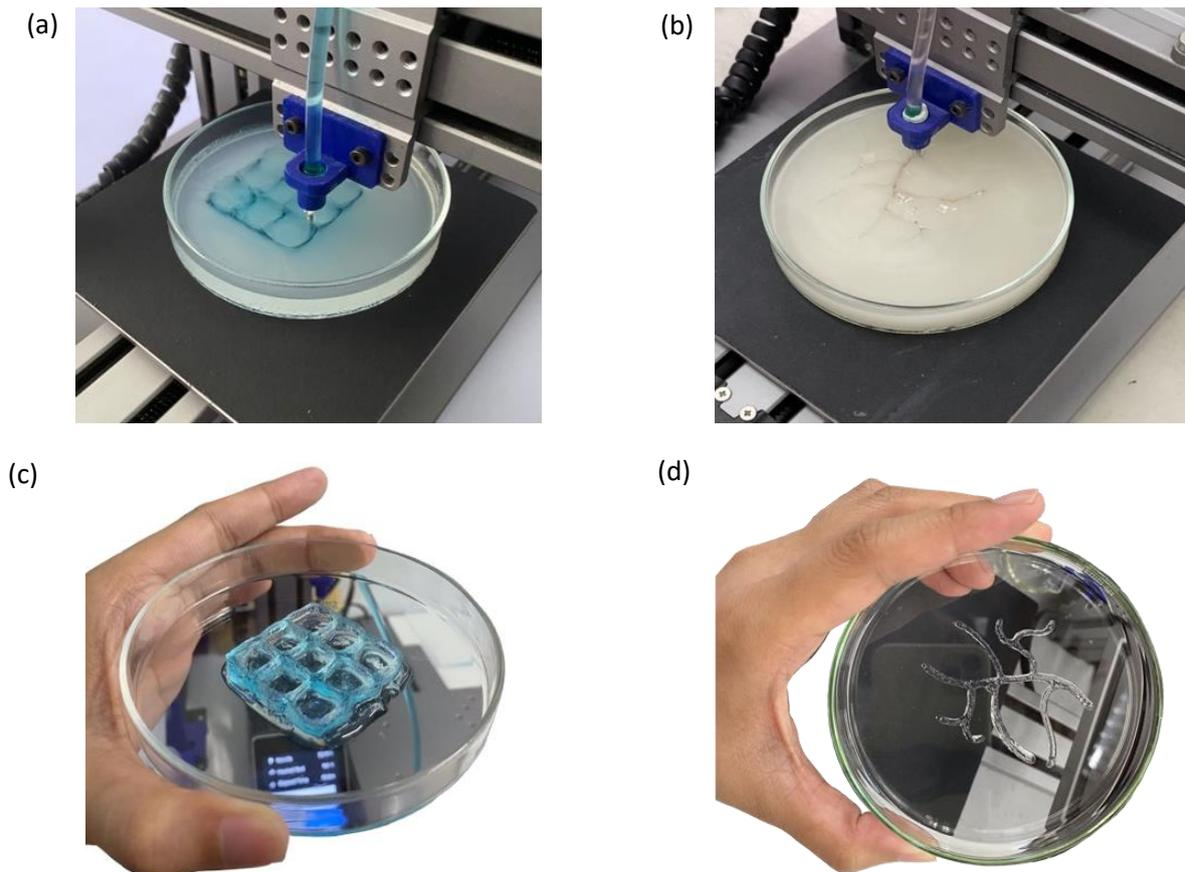
**Fig. 5.** Bioprinting alginate using GelPrint Scaffold method (a) grid square, (b) blood vein profile, 3D printed scaffolds (c) grid square, and (d) blood vein profile
