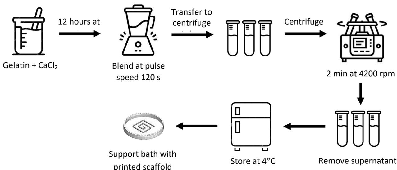
**Fig. 2.** Preparation of gelatin slurry support bath
