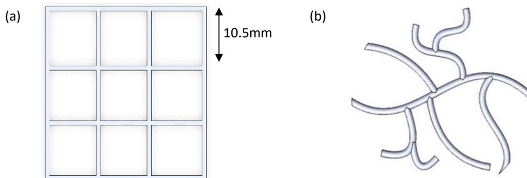
**Fig. 3.** Scaffold designs: (a) grid square, (b) blood vein profile
