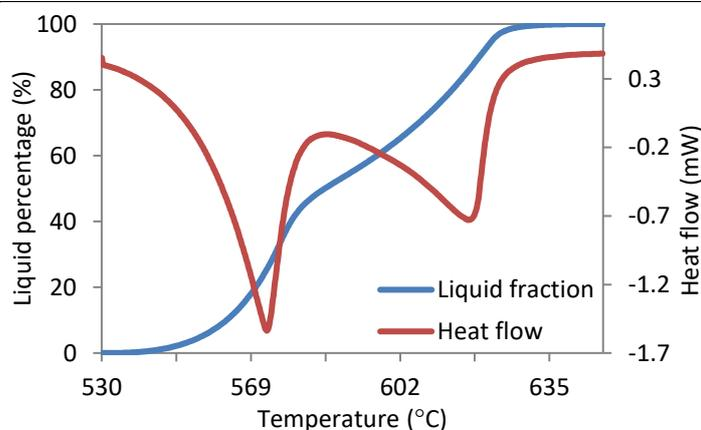
**Fig. 1.** DSC curve of LM4 Al Alloy
