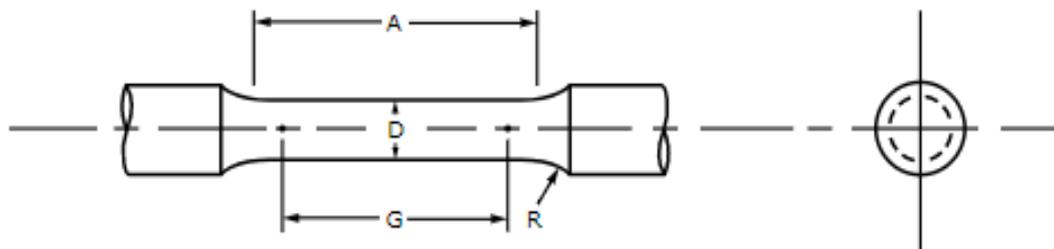
**Fig. 3.** Small-size Specimen Proportional to the Standard Specimen
