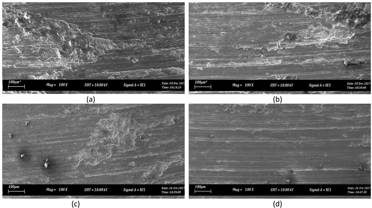
**Fig. 10.** Deformation through dry sliding of LM4 Al Alloy (a) As-cast, (b) CS casted, (c) Thixoformed, and (d) T6-thixoformed sample
