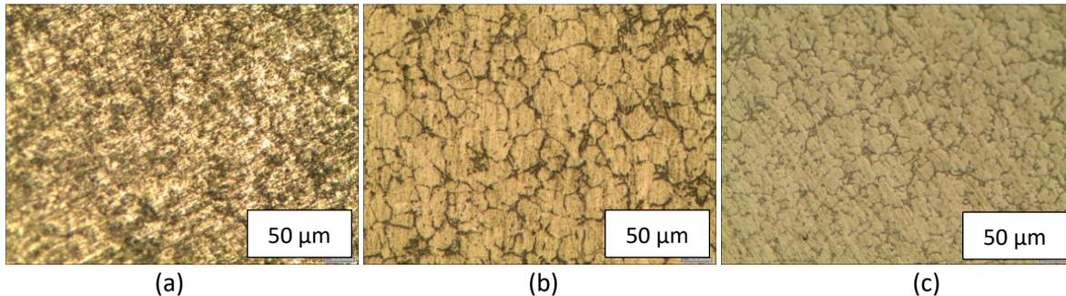
**Fig. 5.** Microstructure of CS casted LM4 alloy at pouring temperature of (a) 620 °C, (b) 640 °C and (c) 660 °C
