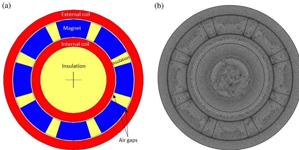
**Fig. 2.** (a) Two-dimensional layout of point absorber structure: iron cores and coils (red), neodymium magnet bars (blue), polymer insulation layers (yellow), and air gap (white), dimension in unit meter; (b) meshing of point absorber structure in COMSOL Multiphysics package
