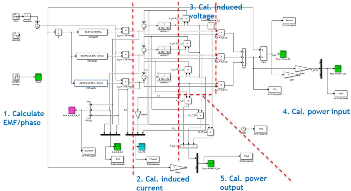
**Fig. 3.** Time-domain based simulation model for point absorber
