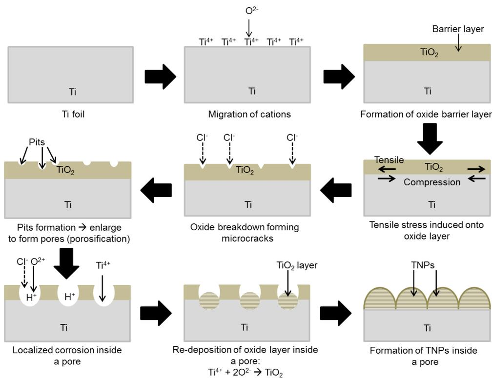
**Fig. 4.** Mechanism of TNPs structure formation in both aqueous and organic electrolytes
