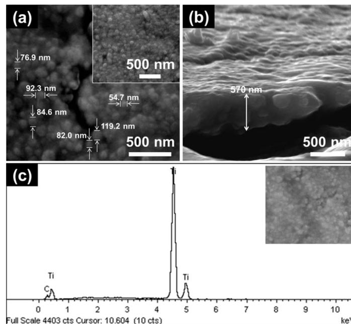
**Fig. 2.** FESEM images of as-anodized sample formed at 20 V for 60 min in 1 M  $\text{Na}_2\text{SO}_4/\text{NH}_4\text{Cl}$  electrolyte: (a) surface morphology (inset: low magnification), (b) cross-sectional view; and EDX analysis (inset: spot area) and (c) EDX analysis of the anodized Ti
