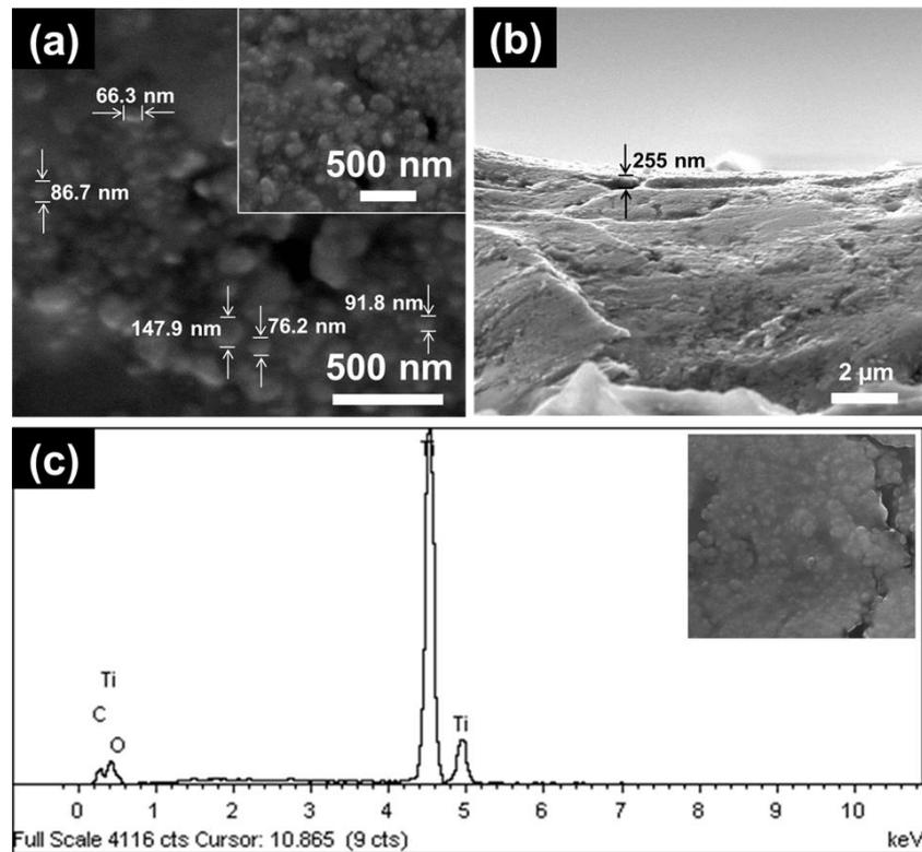
**Fig. 3.** FESEM images of as-anodized sample formed at 20 V for 60 min in glycerol/ $\text{NH}_4\text{Cl}/\text{H}_2\text{O}$  electrolyte: (a) surface morphology (inset: low magnification), (b) cross-sectional view; and EDX analysis (inset: spot area) and (c) EDX analysis of TNPs
