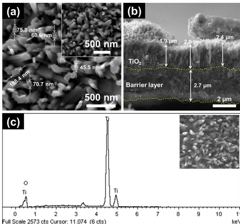
**Fig. 5.** FESEM images: (a) surface morphology (inset: low magnification) and (b) cross-sectional view); and (c) EDX analysis (inset: spot area) of annealed TNPs at  $700^\circ\text{C}$  for 3 h in air fabricated in 1 M  $\text{Na}_2\text{SO}_4$  electrolyte at 20 V for 60 min
