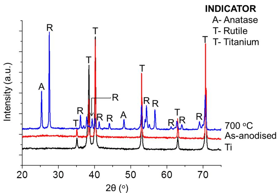
**Fig. 6.** XRD patterns of Ti foil, as-anodised and annealed TNPs at  $700^\circ\text{C}$  for 3 h in air fabricated in 1 M  $\text{Na}_2\text{SO}_4$  electrolyte at 20 V for 60 min
